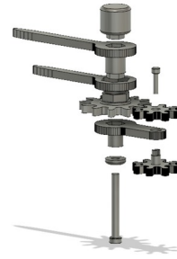
Fig. 7: Multi-part assembly task. In this assembly, parts need to be sequentially grasped and fit together.
